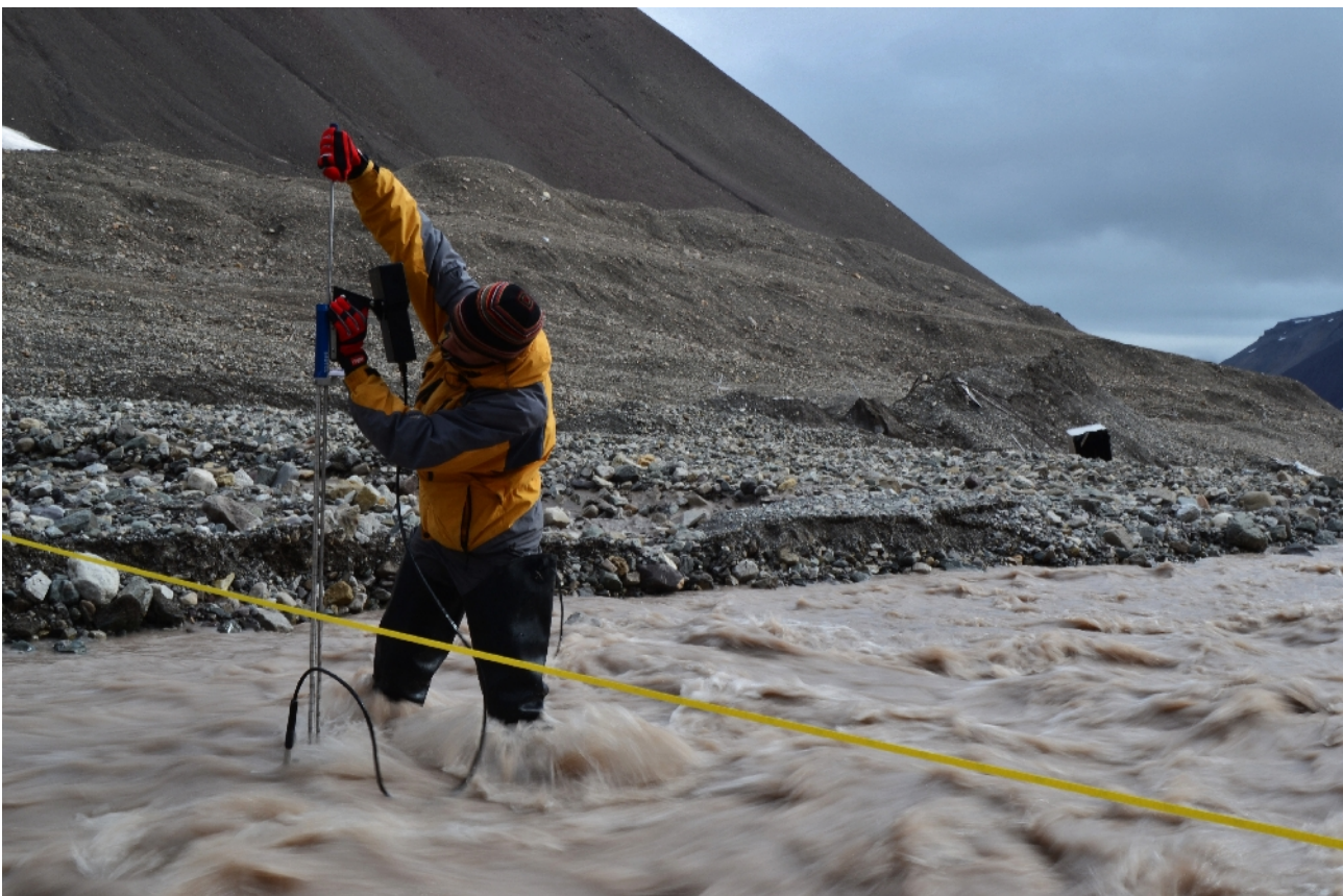
Figure 11. Discharge measurement in the Bertil glacier catchment.
